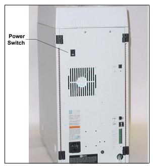
Press the power switch on the ICS-1000 rear panel (see <u>Figure 3-3</u>) to turn on the system power. <u>Table 3-2</u> shows the ICS-1000 conditions at power up.
