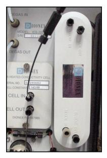
Figure B-20. Suppressor Installed (SRS Shown)
