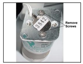
Figure 5-17. Removing the Valve Mounting Plate
