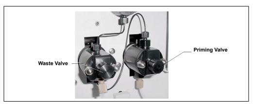
Figure 4-2. Waste and Priming Valves
