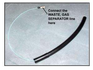
Figure B-21. Gas Separator Waste Tube Assembly
