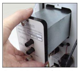
Figure 5-10. Removing the Cell Assembly
