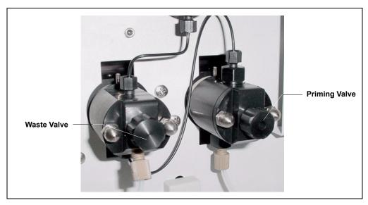
Figure 5-7. Waste and Priming Valves
