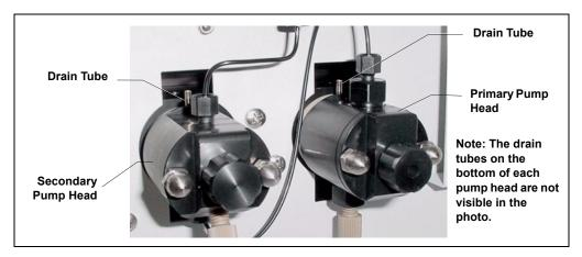
Figure B-47. Primary and Secondary Pump Heads with Drain Tubes
